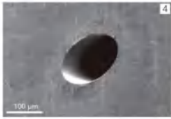
图 1 的细节: 椭圆孔, 长 190 \mu\text{m} , 宽 110 \mu\text{m} (SEM 图像) Detail of figure 1: Elliptical bore hole, 190 \mu\text{m} long, 110 \mu\text{m} wide (SEM image)
