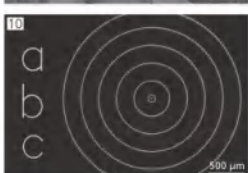
标记图案 - 字符: 0.5 毫米字体, 字体: SimpleStraight3 - 圆形直径: 0mm, 0.1mm, 0.5mm, 1.0mm, 1.5mm, 2.0mm, 2.5mm Marking pattern for labeling - Characters: 0.5 mm font size, SimpleStraight3 font - Circle diameters: 0 mm, 0.1 mm, 0.5 mm, 1.0 mm, 1.5 mm, 2.0 mm, 2.5 mm
