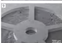
垂直切割的切割应用, 边缘轮廓采用 200 \mu\text{m} 厚的黄铜 (SEM 图像) Cutting application with perpendicular cutting edge contour in 200- \mu\text{m} thick brass (SEM image)
