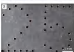
300 \mu\text{m} 厚钢中的 200 \mu\text{m} 钻孔 (入口侧), 通过工件制造, 用 XY 平移台定位 (SEM 图像) 200- \mu\text{m} bore holes in 300- \mu\text{m} thick steel (entrance side), fabricated via workpiece positioning with an XY translation stage (SEM image)
