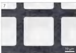
4 x 4 方孔阵列的细节在陶瓷中 - 方形几何尺寸: 30 \mu\text{m} x 30 \mu\text{m} - 深度: 300 \mu\text{m} - 长宽比: 1:10 - 垂直壁轮廓 - 圆角半径: < 4 \mu\text{m} - 壁厚: 10 \mu\text{m} (SEM 图像) Detail of a 4 x 4 square hole array in ceramic - Square geometry: 30 \mu\text{m} x 30 \mu\text{m} - Depth: 300 \mu\text{m} - Aspect ratio: 1:10 - Perpendicular wall contour - Corner-rounding radius: < 4 \mu\text{m} - Wall thickness: 10 \mu\text{m} (SEM image)
